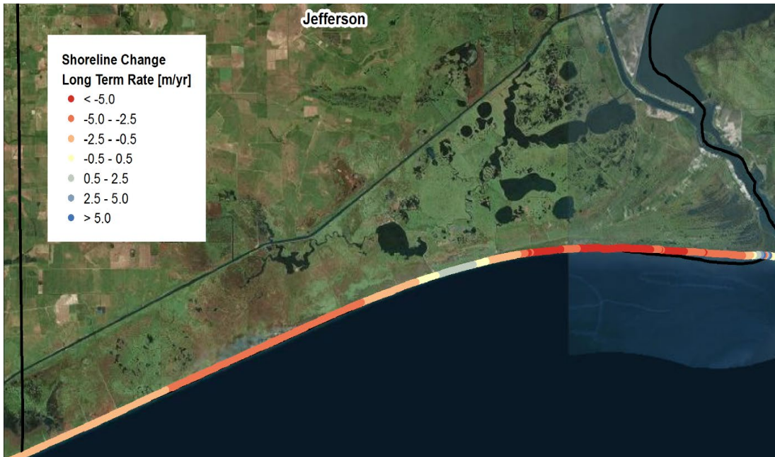
Figure 2-4: Long-term shoreline change rate through Jefferson County, Texas (1930 through 2012)
